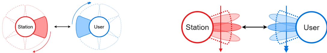
Figure 3: Illustration of a two-stage hierarchical beam search algorithm in azimuth plane. (Left: Exhaustive sector beam search. Right: Ensuing beam refinement using pencil beams.)
