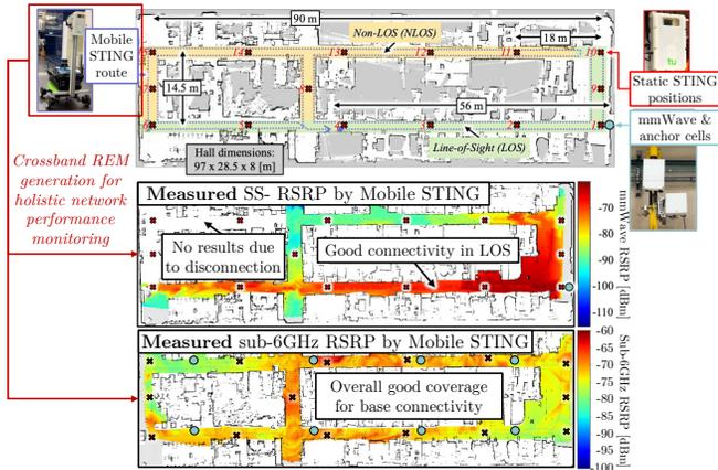
Fig. 11. Crossband KPI Monitoring & Control deployment for mmWave system at Fraunhofer IPT [20]
