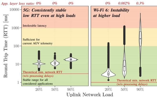
Fig. 10. Comparison of 5G and Wi-Fi RTT with increasing network load
