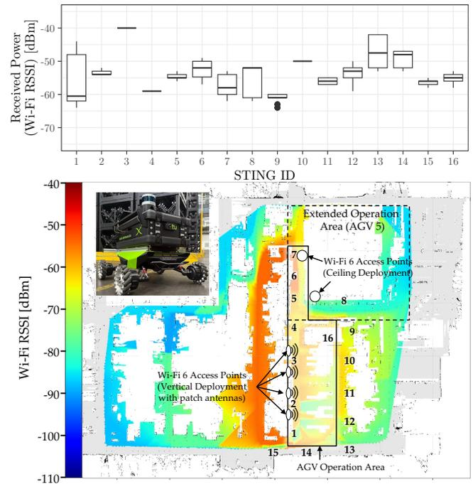
Fig. 8. Radio environmental map of Wi-Fi coverage of AGV operation area
