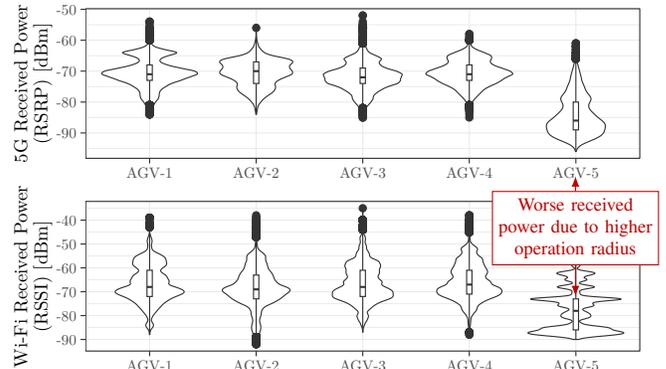
Fig. 9. Comparison of AGV connectivity with deployed 5G and Wi-Fi 6 networks during one exemplary work day
