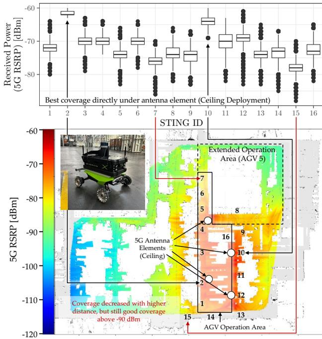
Fig. 7. Radio environmental map shows excellent 5G coverage of AGV operation area
