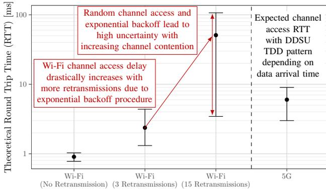
Fig. 6. Theoretical RTT for different number of retransmissions in Wi-Fi compared to channel access RTT in 5G (not considering processing delays)
