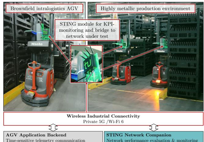
Fig. 1. Intralogistics AGV retrofit with STING unit for 5G and Wi-Fi 6 connectivity and performance evaluation
