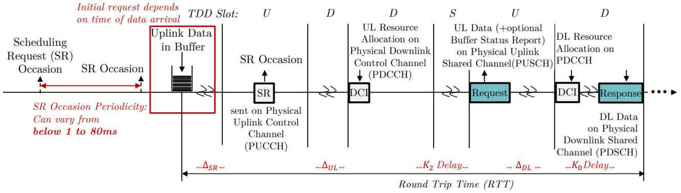
Fig. 5. Minimum Round Trip Time for Request/Response application type in 5G TDD networks
