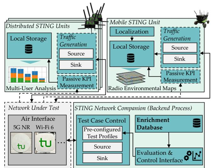
Fig. 2. Overview of STING system architecture
