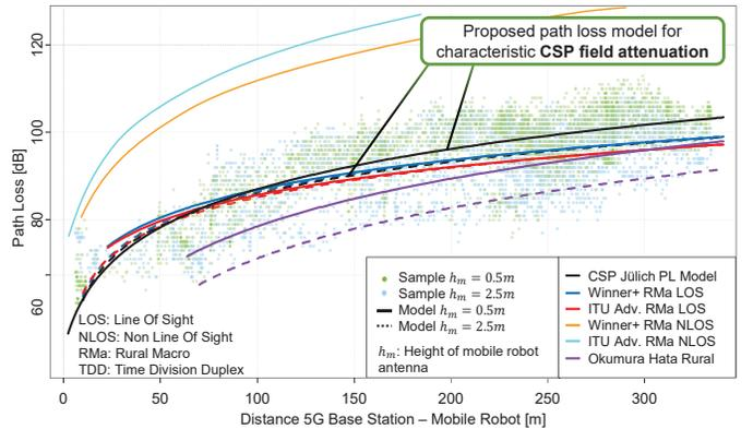
(b) Measurement results to derive channel models for heliostat fields.
