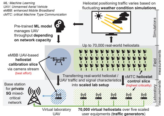
Fig. 1: Multi-dimensional evaluation setup for mixed-critical communication links in lab and field measurements.
