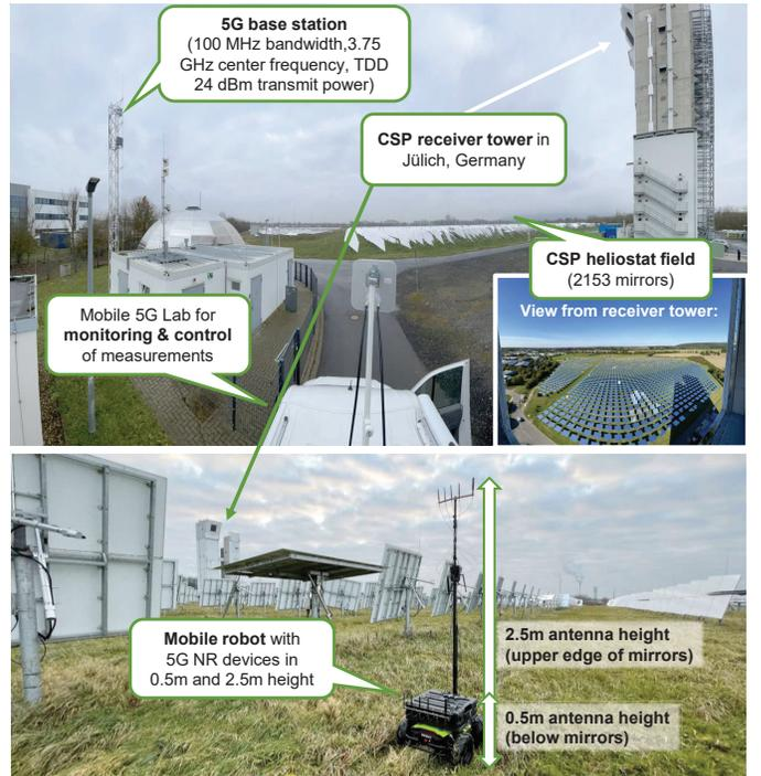
(a) Field measurement setup in CSP plant Jülich, Germany.
