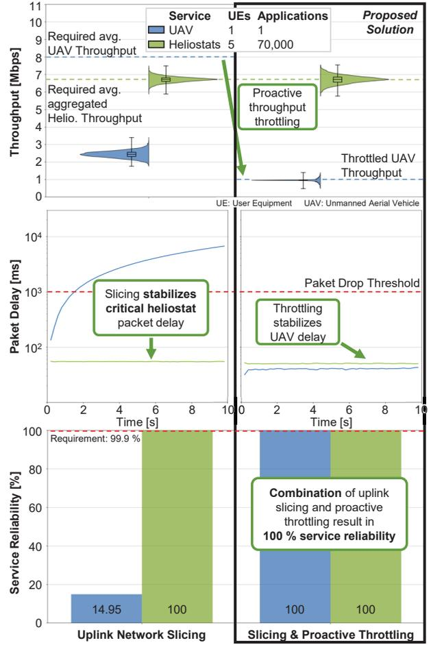
(b) Network Slicing ensures 100 % reliability for the prioritized heliostat traffic. Proactive UAV throttling stabilizes the video stream for UAV control even under worst-case conditions.
