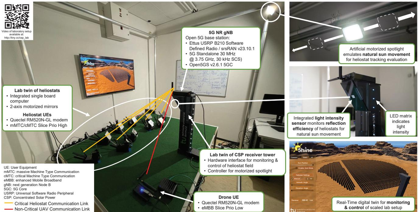
Fig. 4: Experimental setup consisting of an open 5G base station at the receiver tower, heliostats and UAV UEs.
