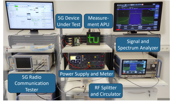
Fig. 3. Laboratory setup to evaluate user equipment power consumption.
