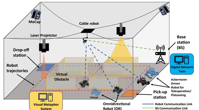
Fig. 5: Testbed setup for scenario evaluation that integrates the proposed system-of-systems architecture.
