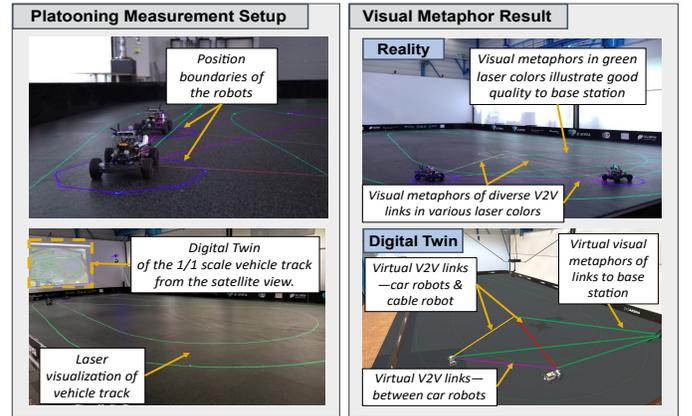
Fig. 9: Platooning measurement setup and the visual metaphor result. The DT illustrates the 1/1 scale of the vehicle track from the satellite view.
