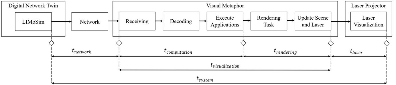
Fig. 4: Overview of the overall system latency contributors based on [20], where the physical network is emulated by the DNT.
