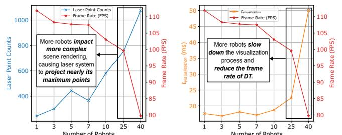
Fig. 7: Frame Per Second (FPS) comparison against laser point counts and FPS comparison against visualization time.
