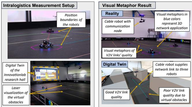
Fig. 10: Intralogistics measurement setup and the visual metaphor result for 3D network management. The DT replicates the Innovationlab research hall and visualizes the virtual obstacles from DNT.
