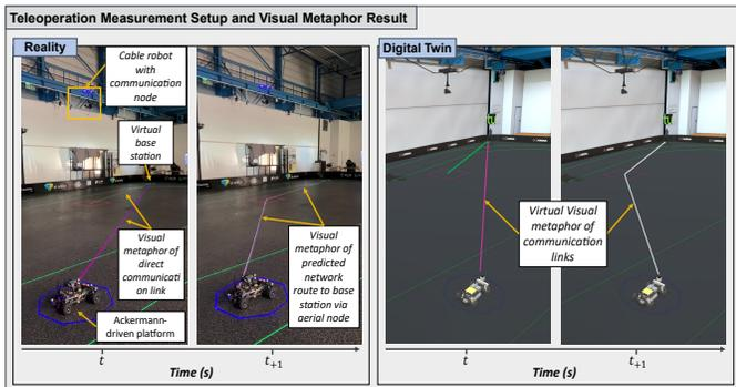
Fig. 8: Teleoperation measurement setup and the visual metaphor result for AI-based network route.
