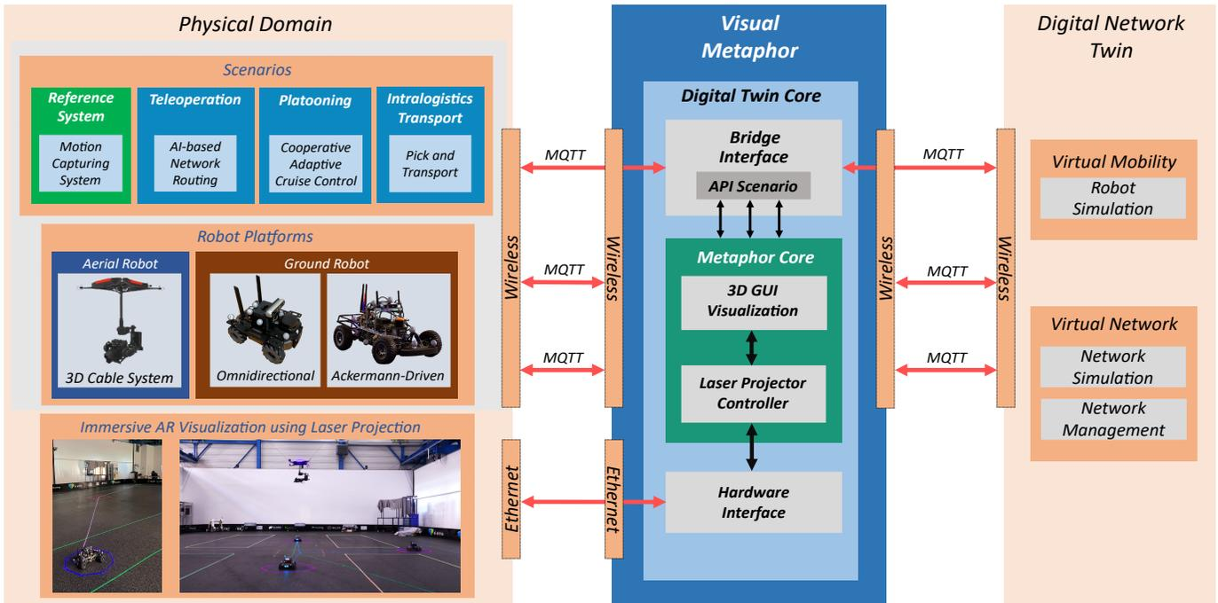
Fig. 1: Proposed plug-and-play system-of-systems architecture for different use-cases including visual metaphor layer. The Message Queuing Telemetry Transport (MQTT) protocol accommodates wireless communication of different systems which are distributed in different locations in the research hall.
