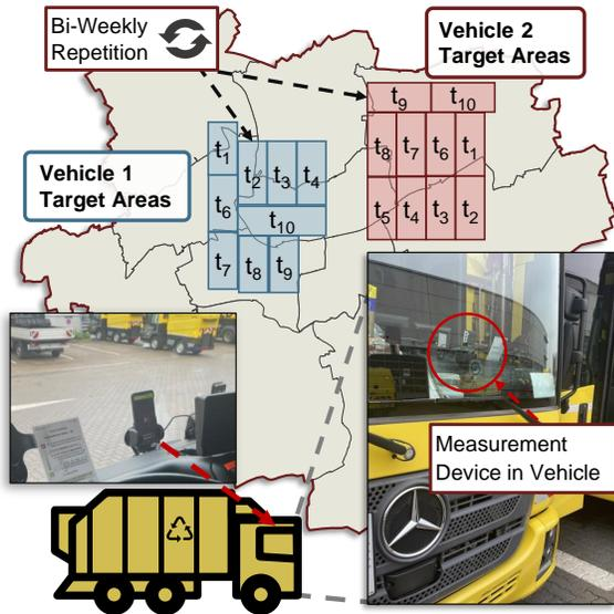
Fig. 3. Measurement device attached to the windshield of a garbage collection vehicle of the Dortmund waste collection company and exemplary repeating daily target areas (Map data: © OpenStreetMap contributors, CC BY-SA).
