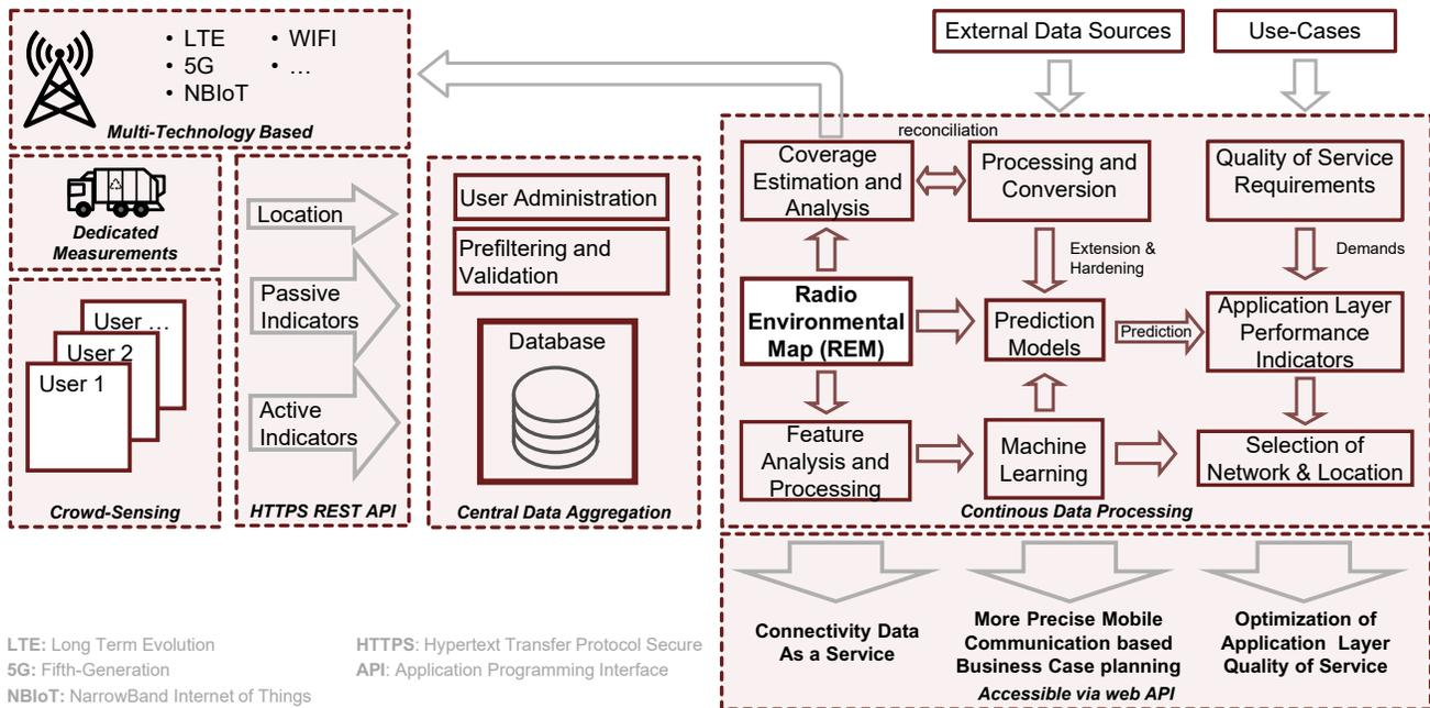
Fig. 2. Developed measurement system used to measure and continuously monitor 5G mobile network performance in the area of the city of Dortmund.
