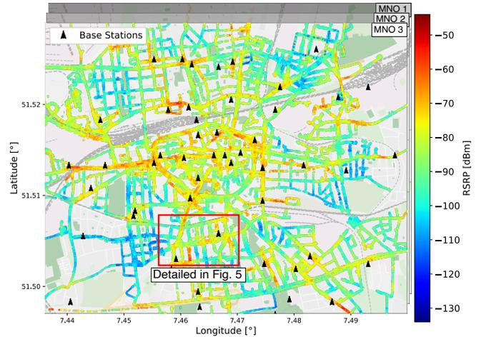
Fig. 4. Scatter plot of the measured Reference Signal Received Power (RSRP) of the first three months of the measurement campaign for Mobile Network Operator (MNO) 3 and base station locations based on openData of the city of Dortmund [17] and the Bundesnetzagentur [9]. The measurement devices are carried on waste disposal vehicles (Map data: © OpenStreetMap contributors, CC BY-SA).
