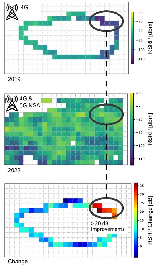
Fig. 6. Comparison of the Reference Signal Received Power (RSRP) REM layer with a cell width of 100 m measured in 2019 by [18] and in 2022 at the Dortmund city ring for Mobile Network Operator 3. It has to be noted that in addition to the RSRP changes, 5G Non-Standalone is available in 2022.
