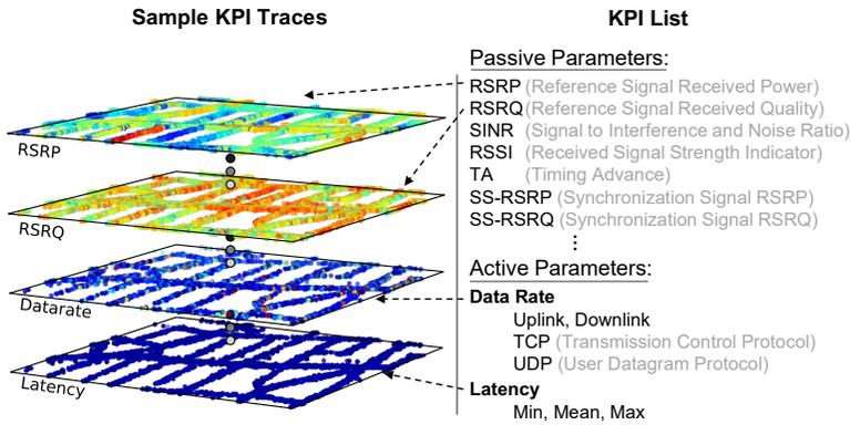
Fig. 5. Selected Radio Environmental Map (REM) layers of measured active and passive Key Performance Indicators (KPIs) for Mobile Network Operator (MNO) 3.
