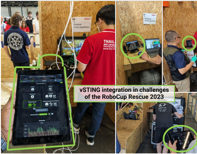
Fig. 2. vSTING during the International RoboCup Rescue 2023 Championship: vSTING was integrated into some arenas of the RoboCup Rescue League and teams that volunteered to challenge their robot’s mobility under network constraints received extra points as a reward.
