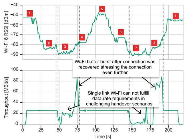
Fig. 5. Data transmissions in the indoor scenario using only the Wi-Fi 6 connect present typical handover situations with occasional decrease in achievable throughput.
