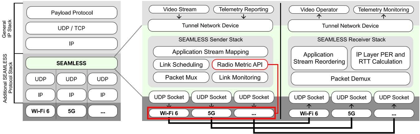
Fig. 2. The Architecture of the proposed SEAMLESS protocol stack, including sender and receiver routines and exemplary payload applications. The approach aggregates multiple radio technologies and utilizes the measured radio metrics for the link scheduling decisions.
