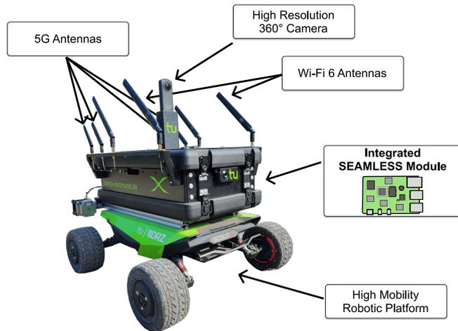
Fig. 3. Photo of the high mobility rescue robotics platform used for the experiments. It is equipped with a high-resolution 360° camera module together with 5G and Wi-Fi 6 connectivity. The SEAMLESS gateway is located in the modular payload housing.
