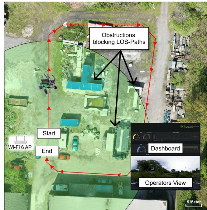
Fig. 8. Experiment in the DRZ outdoor scenario using a locally deployed Wi-Fi 6 AP network and a public 5G infrastructure. A reproducible trajectory was chosen with multiple NLOS situations.
