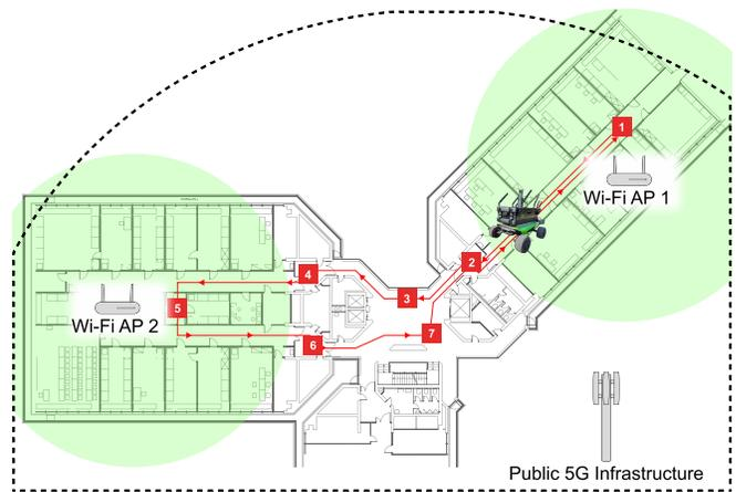
Fig. 4. Indoor evaluation scenario consisting of two Wi-Fi AP and public 5G infrastructure. Additionally, the red line highlights the trajectory of the mobile robotic system.
