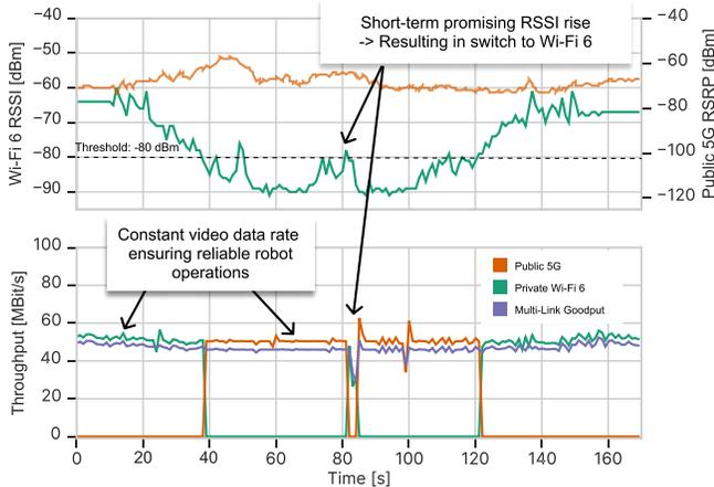
Fig. 9. Radio link aware multi-link measurements in the DRZ scenario transmitting a high-resolution 360° video feed with an average data rate of 50 Mbps. The multi-link Wi-Fi handover threshold is set to  $-80$  dBm. A screen capture of the operator’s video can be found here<sup>1</sup>.
