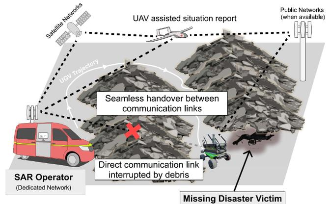
Fig. 1. Presenting a multi-connectivity robotic SAR mission for a missing person, assisted by a UAV-based situation reporting. In challenging radio conditions, where the primary communication link is obstructed, the UGV seamlessly switches to a secondary link.
