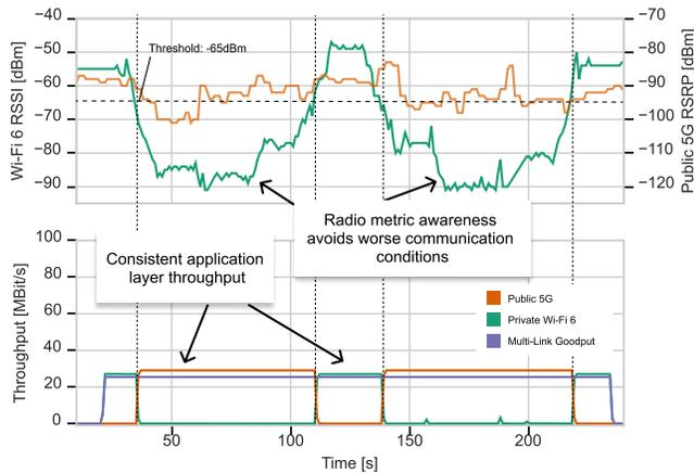
Fig. 6. Multi-link enabled payload data transmission over Wi-Fi 6 and 5G in the indoor inspection scenario. The sender's data rate is fixed to 25 Mbps UDP traffic.
