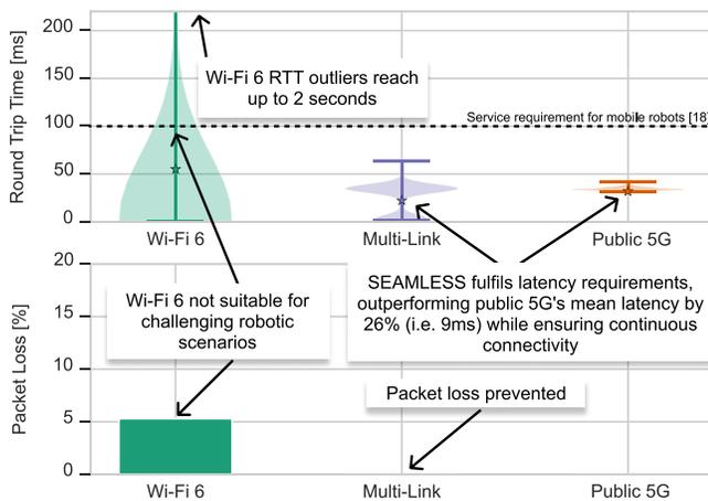
Fig. 7. RTT and PER comparison of SEAMLESS with both Wi-Fi 6 and public cellular 5G in the indoor inspection scenario. Indicating the benefits of the multi-link approach compared to the individual technologies. Note that "\*" represents the RTT mean.
