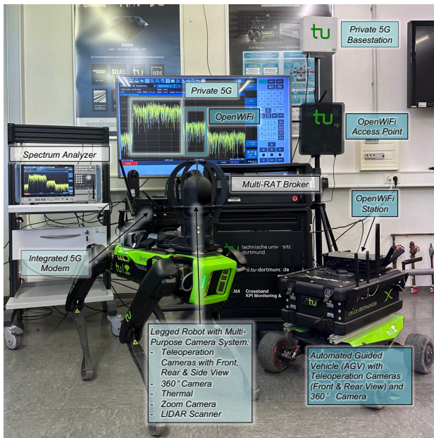
Fig. 3. Experimental setup for OpenWiFi and private 5G coexistence in the 3.7 GHz band
