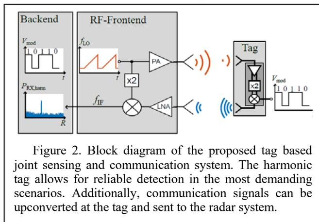
Figure 2. Block diagram of the proposed tag based joint sensing and communication system. The harmonic tag allows for reliable detection in the most demanding scenarios. Additionally, communication signals can be upconverted at the tag and sent to the radar system.
