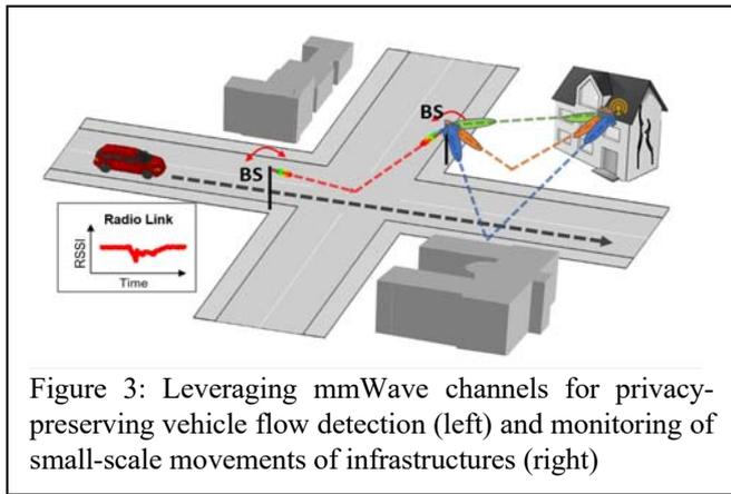
Figure 3: Leveraging mmWave channels for privacy-preserving vehicle flow detection (left) and monitoring of small-scale movements of infrastructures (right)
