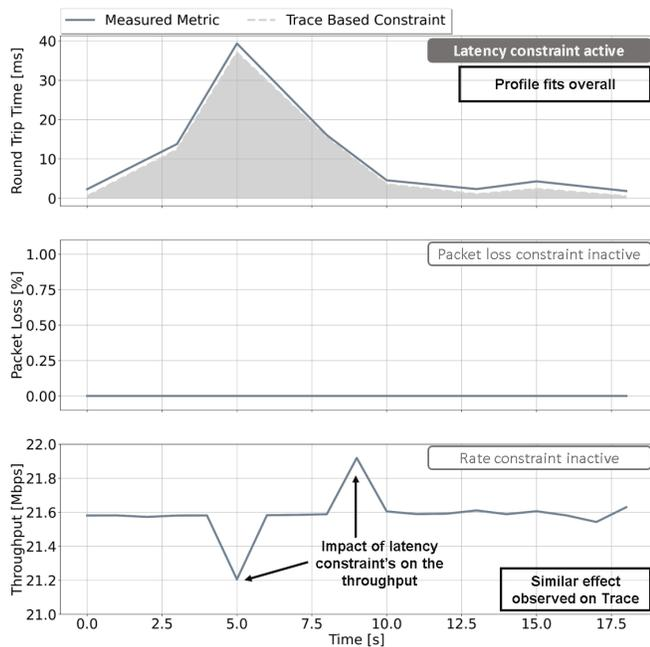
Fig. 9. Network replay while using only the latency traces as constraints. The generated metrics for the latency match the recorded trace profile. The throughput shows a similar trend to the traces in response to latency fluctuations.
