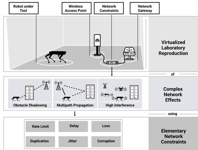
Fig. 1. The envisioned approach for evaluating robotic applications under realistic connectivity conditions: leveraging simple network constraints through network emulation to rebuild complex network effects on live traffic.
