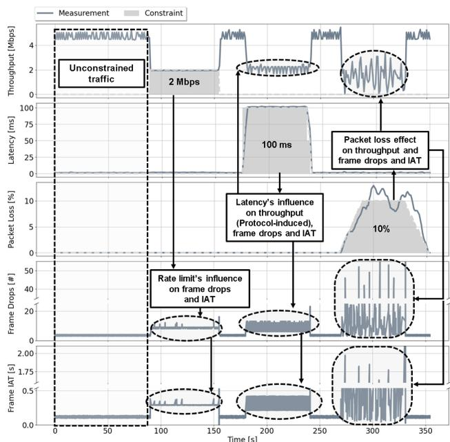
Fig. 5. Manual enforcement of constraints on live traffic of a robot’s FPV Camera. The physical dependencies between the network metrics and protocol-induced cross-metrics effects can be observed. Frames drops and Inter Arrival Time (IAT) also monitored, to capture the constraints’ effect on the FPV stream.
