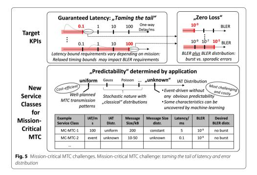
URLLC requirements with its envisaged target KPI values of a latency bound of 0.1 ms combined with block error rate (BLER) of  $10^{-9}$ .
