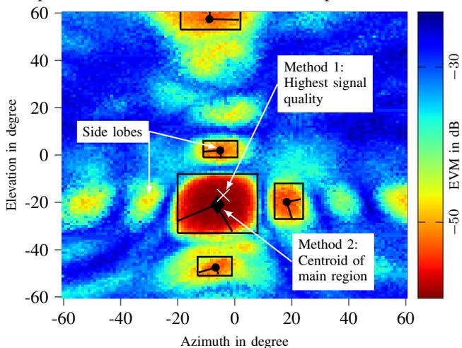
Fig. 5. Heat map of measured EVM of DM-RS as signal direction quality indicator of one exemplary exhaustive sweep. The direction estimates determined by the two proposed methods are marked as white cross and black diamond respectively and could be considered as bearing direction for subsequent cross-bearing positioning.
