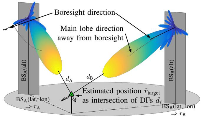
Fig. 2. Cross-bearing as a basic principle of the proposed positioning. The intersection (or its least squares approximation) of at least two base station DFs (denoted as  $d_i$ ) embodies the estimated mobile device position. The base station positions  $r_i$  and orientations are assumed as given for the computation.
