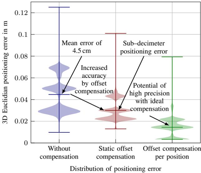
Fig. 7. Statistical evaluation of achieved positioning performance using the second proposed DF method. Compensation is applied in post-processing to account for the mean angular offset in total and individually per mobile device position, respectively.
