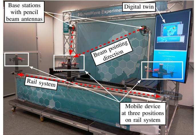
Fig. 4. Laboratory setup for experimental evaluation. The pencil beams of two phased array antennas are directed towards the mobile device at the three indicated positions.
