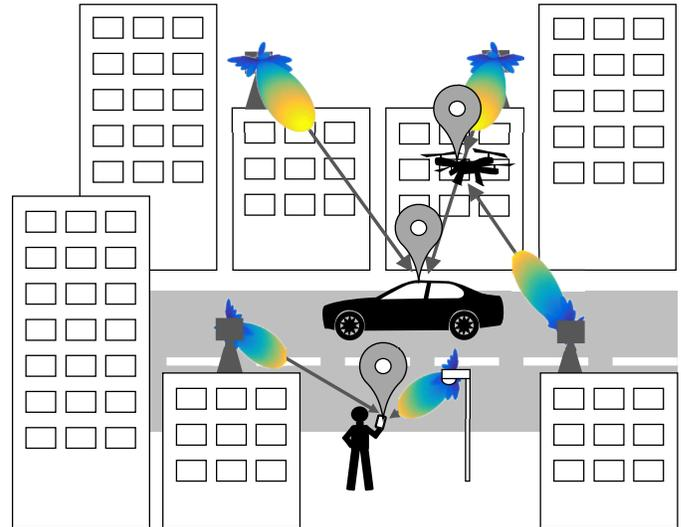
Fig. 1. In the exemplary context of road traffic, pedestrians, motor vehicles and Unmanned Aerial Vehicles (UAVs) as 5G mobile network subscribers may benefit from a mmWave–based positioning service, realizable by exploiting beam alignment information as bearing.
