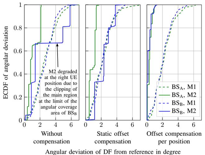
Fig. 6. ECDF of the achieved DF precision in terms of the angular deviation from reference pointing directions of both antennas  $BS_A$  and  $BS_B$  and the two discussed estimation methods M1 and M2. The precision is slightly increased by static offset compensation and further enhanced by an individual offset compensation per UE position. Especially the centroid method (M2) performs well with a maximum deviation of  $1.38^\circ$ .
