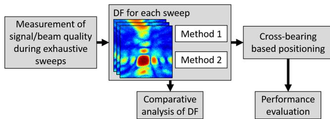
Fig. 3. Methodology of experimental evaluation. Based on the measurement results, DF is computed with the described methods. Finally, the target position is estimated by cross–bearing and the performance is evaluated.
