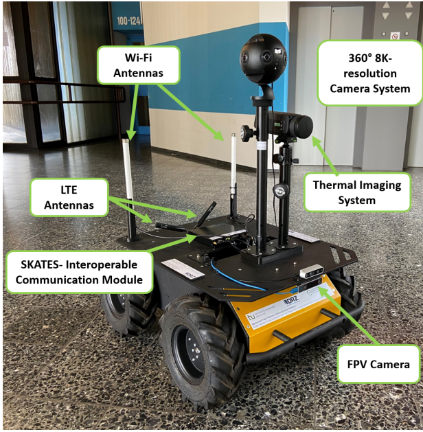
Fig. 5. Photo of the evaluation equipment shows the Husky SAR robot. On top of the Husky, the communication equipment (the interoperable communication module with an LTE-Modem and Wi-Fi configuration) are attached. The 360° camera is also mounted on top, using a stand.
