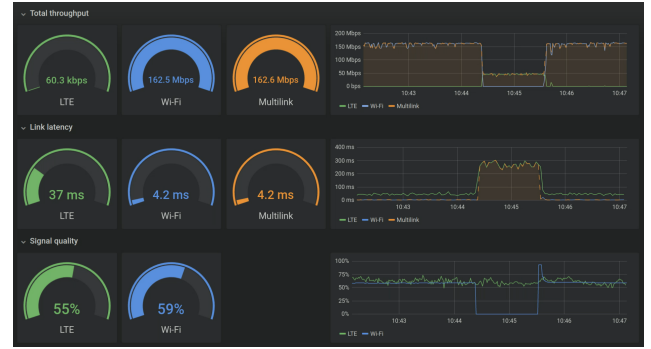
Fig. 4. The communication dashboard of the health monitoring in the SKATES backend shows the key-performance indicators throughput, latency and signal quality for the individual interfaces as well as for the combined multi-link.
