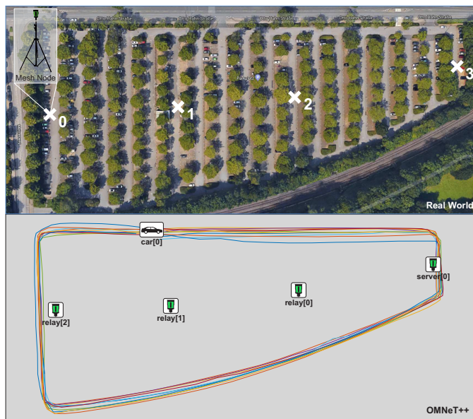
Fig. 4. Overview of the field test scenario and its representation within the OMNeT++ simulator for the validation.
