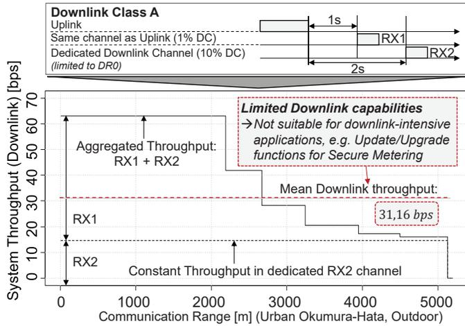
Fig. 4: System Throughput (Downlink) utilizing maximum duty cycle capabilities
