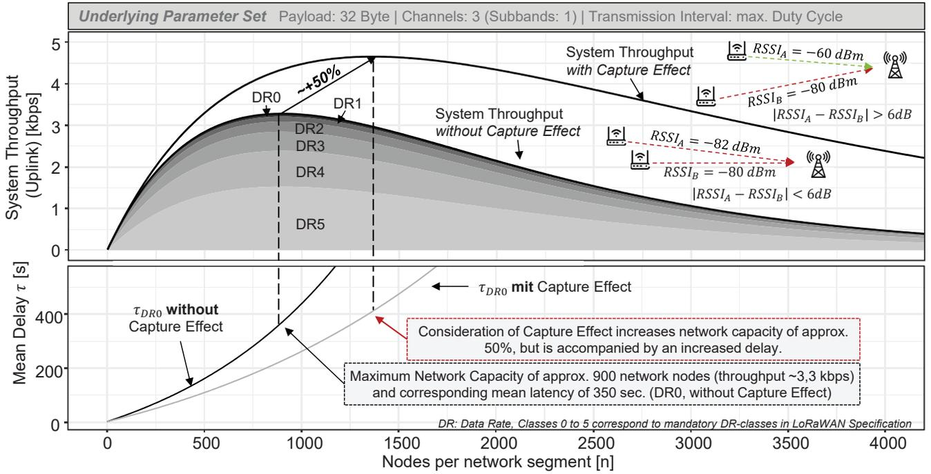
Fig. 5: System Throughput (Uplink) and Latency utilizing maximum duty cycle capabilities
