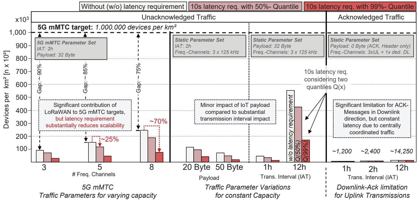
Fig. 7: Impact of various LoRaWAN parameter configurations on maximum scalability considering 5G mMTC connection density and latency requirements
