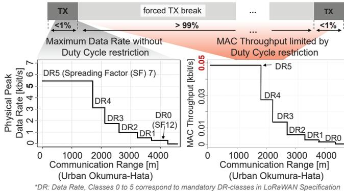
Fig. 2: Impact of regulatory duty cycle restrictions on LoRaWAN data rates
