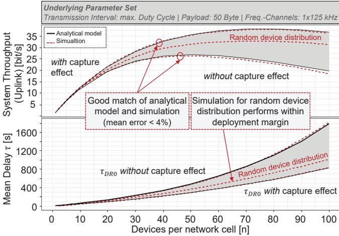
Fig. 6: Validation of analytical model through LoRaWAN network simulation using OMNeT++
