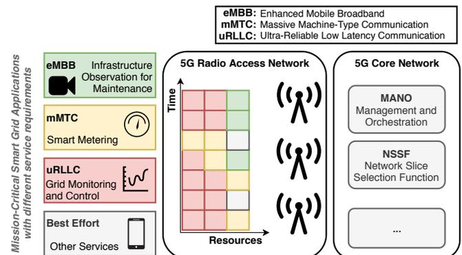
Fig. 1. End-to-end 5G Network Slicing architecture with example mission-critical Smart Grid applications.
