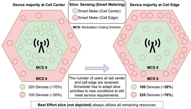
Fig. 7. Slice configuration and measurement procedure of Scenario 2, split into a situation with the majority of devices at cell center (left) and another one with the majority of devices in cell edge (right), both containing high-priority Smart Metering devices.
