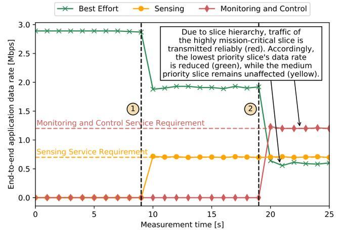
Fig. 6. Measurement results of inter-slice resource sharing in the *critical* operation state of slice *Monitoring and Control*. As the *Sensing* slice (yellow) has a higher priority than the non-critical *Best Effort* (green), data rate needed for the high-priority slice is deducted from *Best Effort* users.
