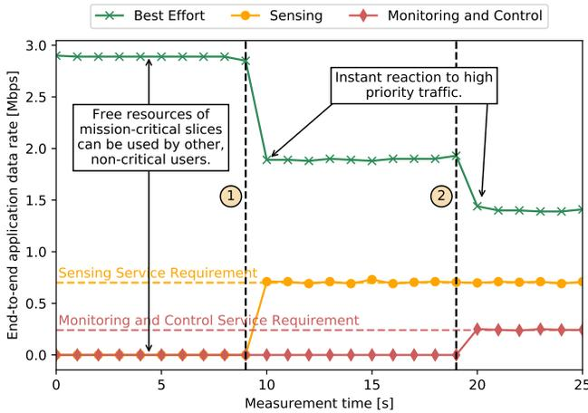
Fig. 5. Measurement results of inter-slice resource sharing in the *normal* operation of the highly mission-critical *Monitoring and Control* slice (red). Unused resources of high-priority slices are efficiently assigned to the next slice in the hierarchy until these resources are needed.
