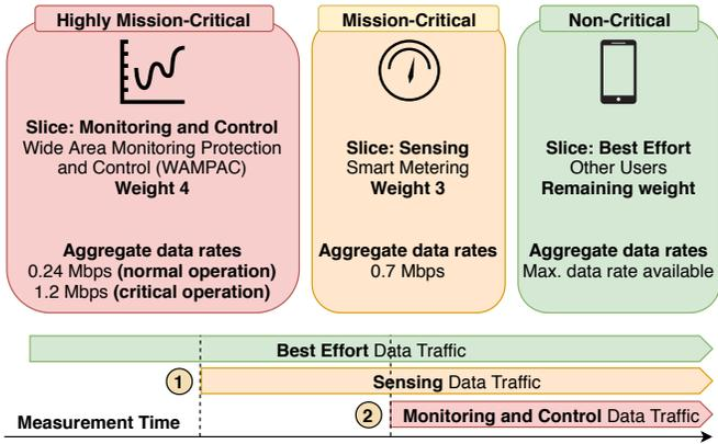
Fig. 4. Network slice configuration and measurement sequence of Scenario 1, split into *normal* and *critical* operation states for the *Monitoring and Control* slice. The goal of this scenario is to show the hierarchical service prioritization and effective inter-slice resource sharing of the implemented Network Slicing scheduler.
