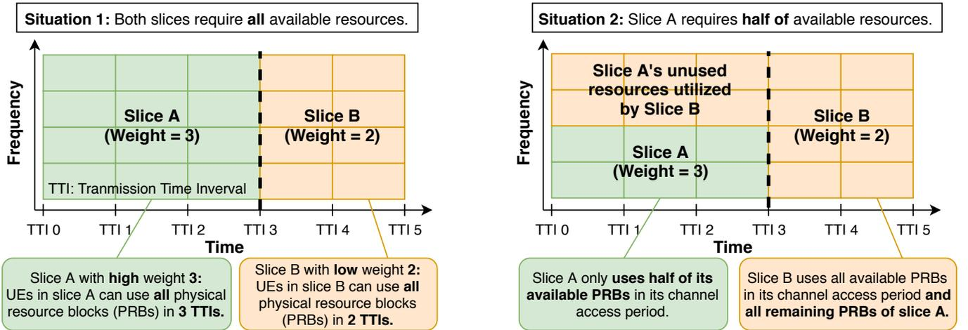
Fig. 2. Example situations showing the operation principle of our proposed and developed scheduler implementing RAN Network Slicing.
