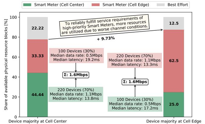
Fig. 8. Measurement results of Scenario 2: The share of PRBs for each slice is shown. As more devices shift to the cell edge (right side), and the required sum data rate of the high-priority *Sensing* (Smart Metering) slice remains unchanged, more PRBs are required to fulfill the same QoS constraints. These are reliably deducted from the non-critical *Best Effort* slice.
