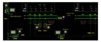
Figure 3: Process visualization of MAS and DPFCs embedded in an exemplary 110 kV grid in PSIcontrol
