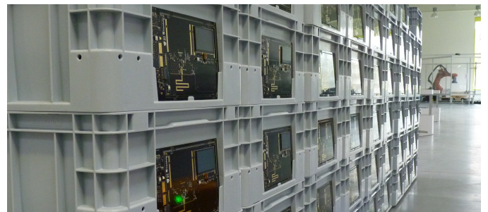
Fig. 1. Photograph of the PhyNetLab, an IoT-based warehouse testbed, which consists of a large-scale deployment of energy-harvesting and communicating smart containers (PhyNodes).
