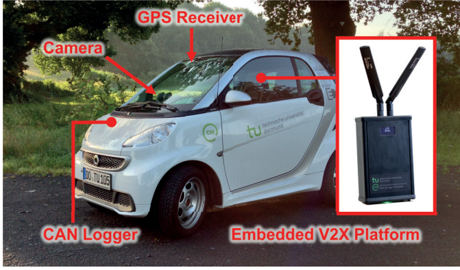
Fig. 2. Research vehicle and car-to-cloud platform that were used for the empirical evaluation
