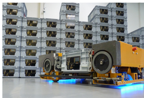
Fig. 1. Photograph of the PhyNetLab , a large logistics hall containing numerous smart containers, each attached with a communicating PhyNode . PhyNetLab serves as a large-scale testbed for the development of future, IoT-based warehouses.
