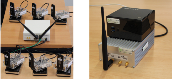
Fig. 5. Left: Measurement setup of the near scenario using an USRP N210 as eNodeB and six STGs including the DUT. Right: LTE passive probe consisting of an USRP B210 and a compact PC executing the modified OAI-software.
